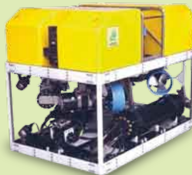
KINGFISHER INSPECTION AND LIGHT WORK-CLASS ROV
